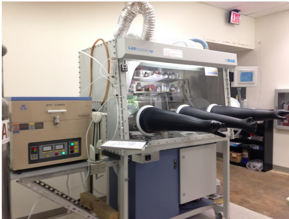
Figure 4. Glovebox and adjacent tube furnace for sample production
