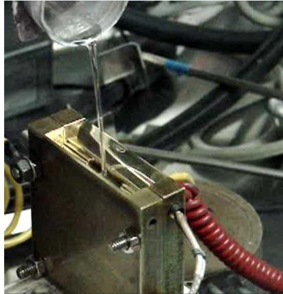
Figure 6. Molten FCZ glass being poured into preheated brass mold.
