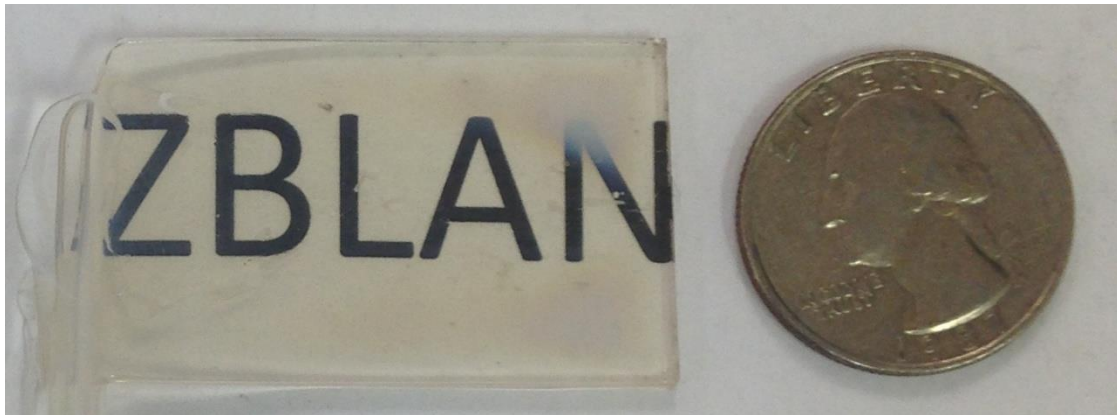
Figure 7. Example of synthesized amorphous glass sample once removed from mold. A quarter is shown for scale.
