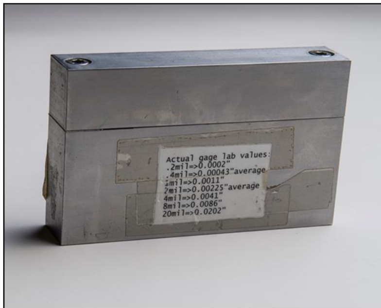
Figure 28. Gap phantom used for CR image testing [30]. Used with permission.
