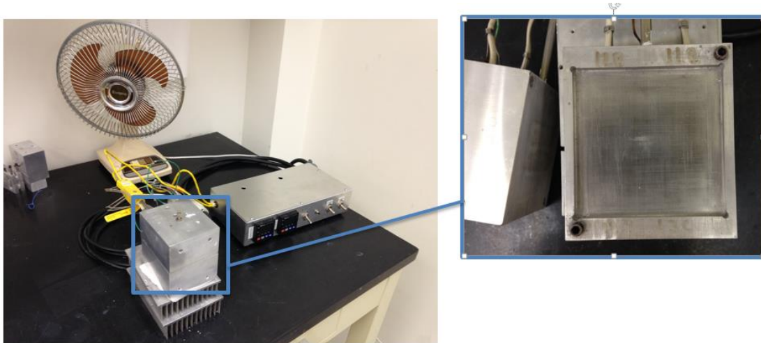
Figure 9. Newer heat treatment system with split aluminum block and separate cartridge heaters and PID controllers
