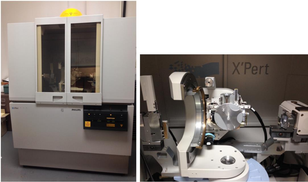
Figure 13. Philips X'Pert XRD used for x-ray diffraction measurements.
